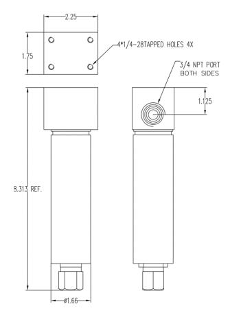
Figure 4. Dimension of the ST-500SS (inch)
