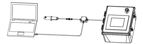
Figure 6. USB connection to ST-500 Series sensor
