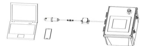
Figure 5. Bluetooth connection to ST-500 Series sensor
