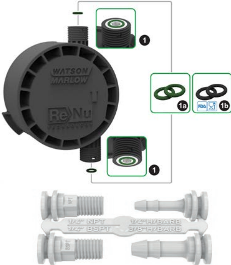
Figure 28 - Connecting interface tubing to a ReNu 30 pumphead
