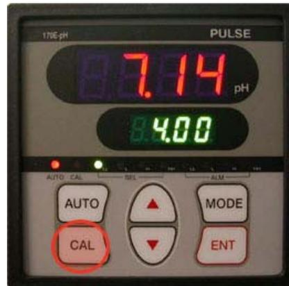
3. The "CAL" indicator light will turn on and the top display will start blinking. The second display will display "4-7" for a few seconds.
