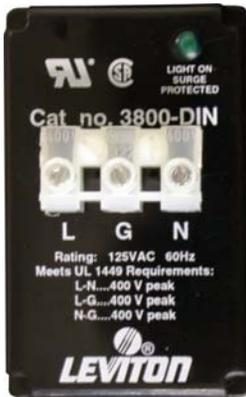
A surge suppressor is used to protect the control panel to prevent damage from loads voltage surges, spikes, and electrical line noise. The green LED on the surge suppressor indicates that the surge suppressor is working. If the green LED is off, this indicates that power is not being supplied to the surge suppressor. In addition, the LED will not illuminate if there has been a utility power failure or a short circuit.
