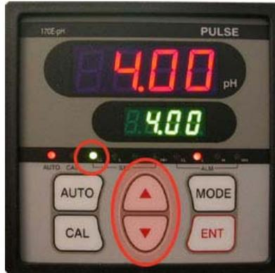
4. Press the “ENT” key to save the set point and the second display will blink rapidly to confirm.
