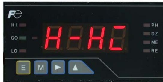
8. Press the “M” button until the display shows “H-Hi” and then press the “M” button again to change the hysteresis value.
