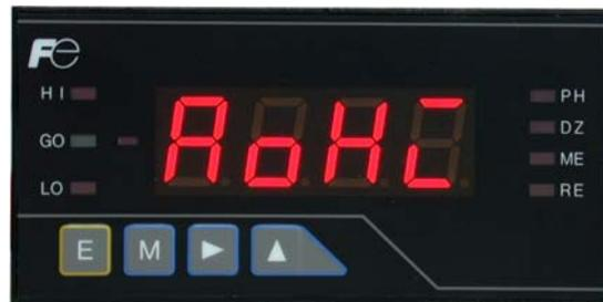
6. Press and hold the “E” and “M” buttons for three seconds. The screen will display “cond”.
