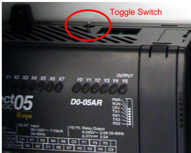
To reset the PLC located on back plate inside of the control panel, toggle the switch to STOP (to the right), then to RUN (to the left without stopping in the middle). Finally, position the toggle switch to TERM (to the middle).
