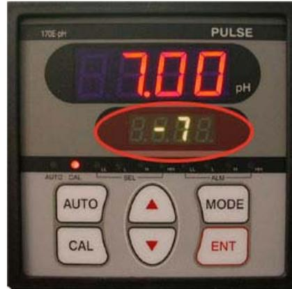
5. Rinse the electrode with water and place it in the pH 4.01 buffer solution and allow sufficient time for the electrode to reach the buffer solution value.
