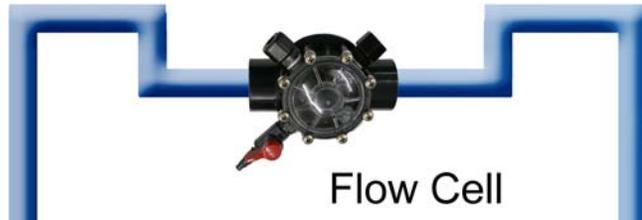
The pipe is in a U-shape to trap water, so that the electrodes will stay wet. For some electrodes, it is essential that they stay wet at all time.
