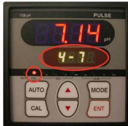
4. The controller will automatically calibrate to the buffer solution value (pH 7.00). The first and second display will stop blinking after the controller is calibrated to pH 7.00. The second display will show “- 7”.
