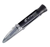
The Mater M series of refractometers are new hand-held refractometers developed with high quality and ease of use in mind. The refraction view is brighter than that of all current models. The prism housing of the Master M refractometer is made of metal allowing for the temperature of hot or cool samples to conform to the temperature of the prism quickly. The Master M series is the successor model to the conventional N-1a.
